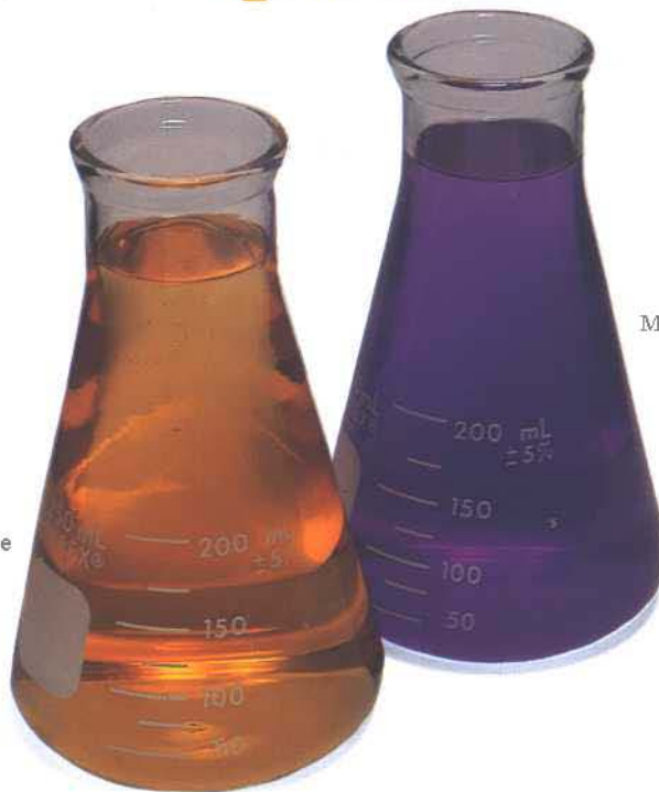
This is a visual demonstration of the color change that takes place when the ME Ultimate spent. The fresh solution is yellow and the spent solution is purple.
